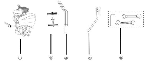
Package: ①Tiller ②Walking Wheels ③Handle Connect Bending Pipe ④Resistance Rod ⑤Tools
